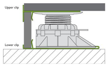
**PROSTILT facing profile in V2A brushed stainless steel** To cover the butt joint at the vertical facing
