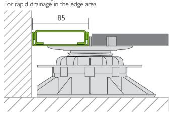
**PROSTILT upper clip / U-Profile lower** To frame and protect the free edges of the flooring
